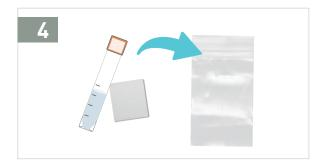
4. Put the sample tube in the protective bag with the cellulose wadding. Then close the protective bag carefully.
