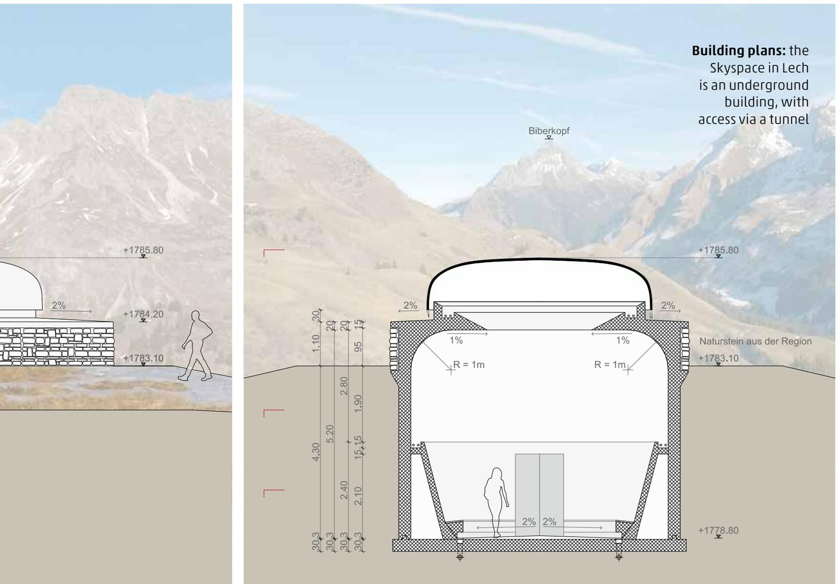
**Building plans:** the Skyspace in Lech is an underground building, with access via a tunnel
